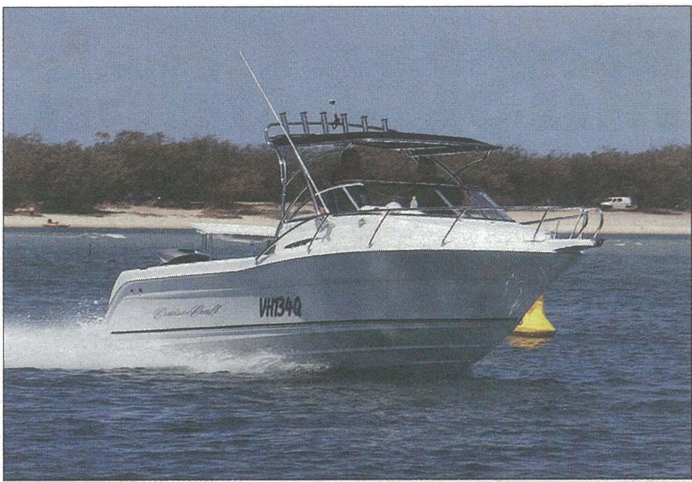
The sharp entry and planing plank provide a soft and dry ride.
